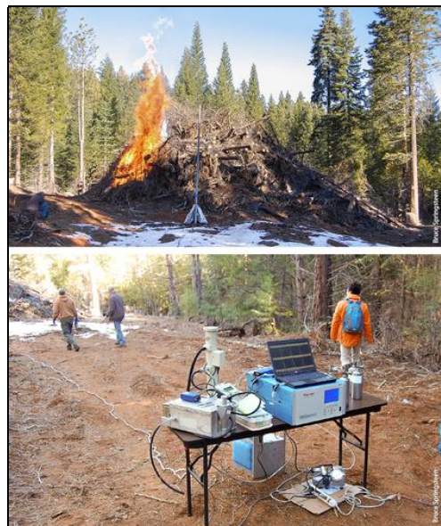
Fig. 2. To sample air emissions from the pile burn, researchers used a 20-foot steel probe at the edge of the pile (top); nitrogen oxides, black carbon and carbon dioxide were measured on site using continuous emissions monitors. Canister samples were collected and sent for off site analysis for total fine particulate matter, trace hydrocarbons and carbon monoxide.
