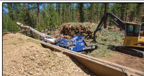
Contractor CTL Forest Management Inc. loads a chip van with woody biomass waste from the Yeti Fuels Reduction Project in the Lake Tahoe Basin Management Unit, Kings Beach, CA. A case study at Blodgett Forest Research Station quantified the air quality and energy benefits of converting biomass waste to electricity as an alternative to open pile burning in the forest.
