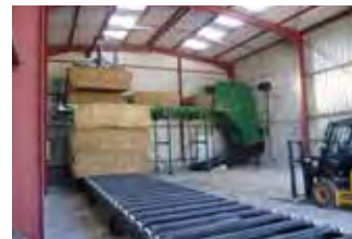
Grass Cutter and Feeding System for cutting and feeding switch grasses, miscanthus, straw, and similar into boilers.
