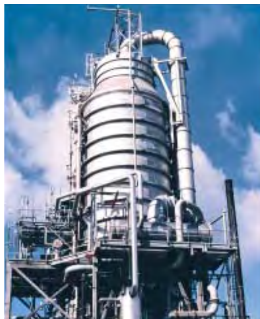
Mechanical booster combined with a DRYFLO type ALLEX dry vacuum pump system for a drying application at
