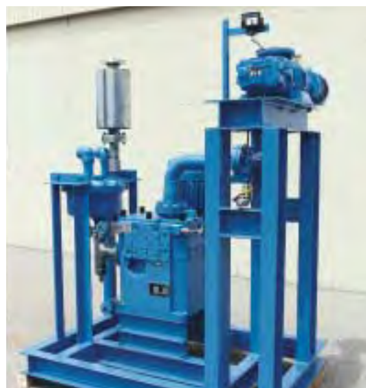
Mechanical booster combined with a DRYFLO type ALLEX dry vacuum pump system for a drying application at
