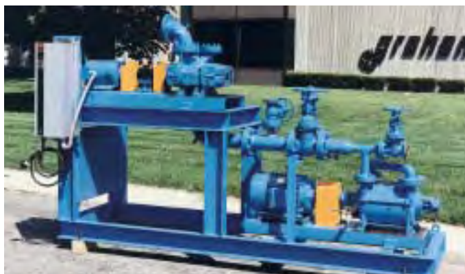
A combination mechanical booster and liquid ring vacuum pump system for a plastics and resins plant in Canada.
